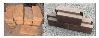
Fig 4: traditional fired brick ISSB brick
